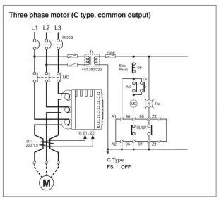
Basic model: EOCR-3DM2 (Z) / FDM2 (Z)
