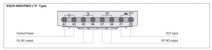
Basic model: EOCR-3DM2 (Z) / FDM2 (Z)
