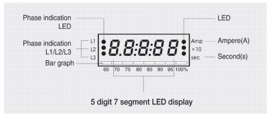
3 phase load currents (In) and a leakage current (i3MZ/iFMZ) are displayed every 2 seconds in sequence.
