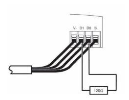
Please use a cable with 2pair shieded twisted conductors for Interface protection. It is adviced to isolate the Modbus cable 30cm(11.8in) at least from a power cable. If necessary, intersect the Modbus cable to a power cable perpendicularly. Refer to the diagram in the left side for the line terminator wiring.
