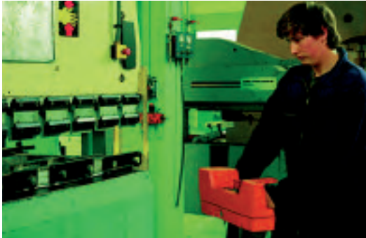
↑ Fig. 28 Two-handed control on a press
