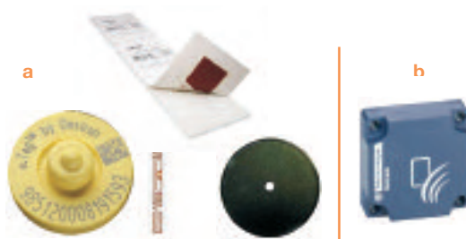
↑ Fig. 32 a et b a - RFID formats designed for different uses b - RFID industrial (Telemecanique Inductel)
