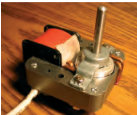
↑ Fig. 10 Single phase short circuit phase-shift rings
