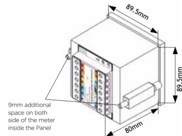
9mm additional space on both side of the meter inside the Panel
